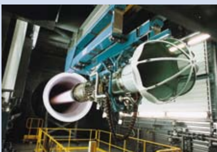
All maintenance work is complete. Testing on the in-house engine test bed
