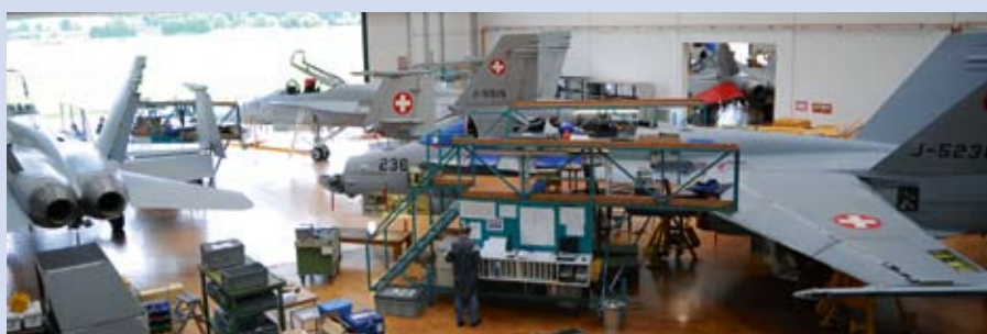
Various components are removed for servicing at the relevant competence centres
