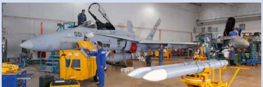
In-depth testing of all systems after completion of servicing
