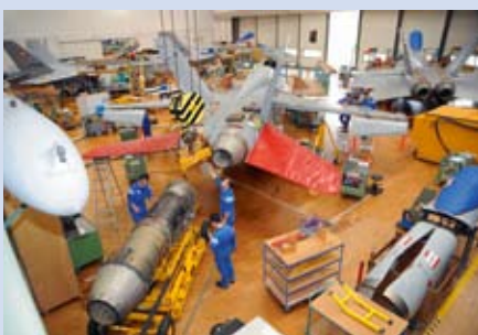
The engines are removed and taken to the competence centre
