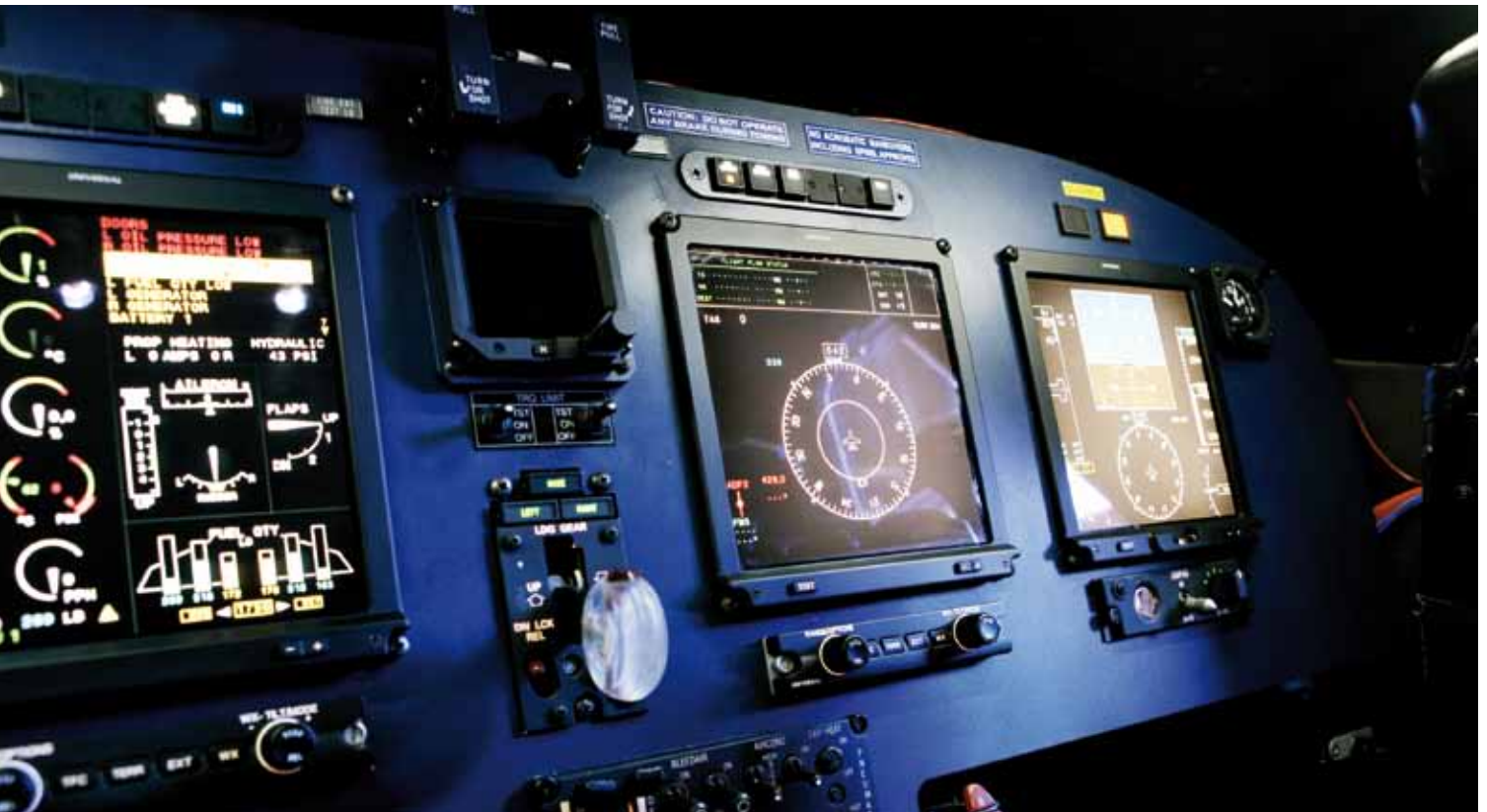
All key flight data at the pilot's fingertips: the innovative glass cockpit and avionics of the Do 228NG.
