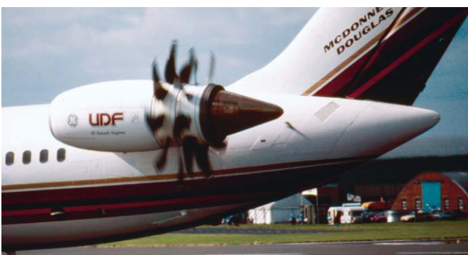
Unducted fan project 1988. Photo courtesy of Pima Air & Space Museum, Tucson, AZ
