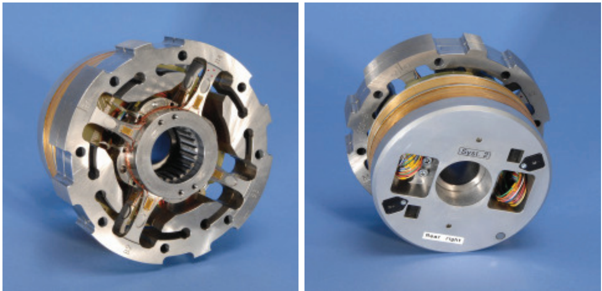
Figure 4. RUAG RSB 320. Fully symmetric spoke-type balance with 2 transversal planes in axial direction each containing 4 spokes. On either side of the inner non-metric part of the balance the transmitter unit of the telemetry system can be attached to.
