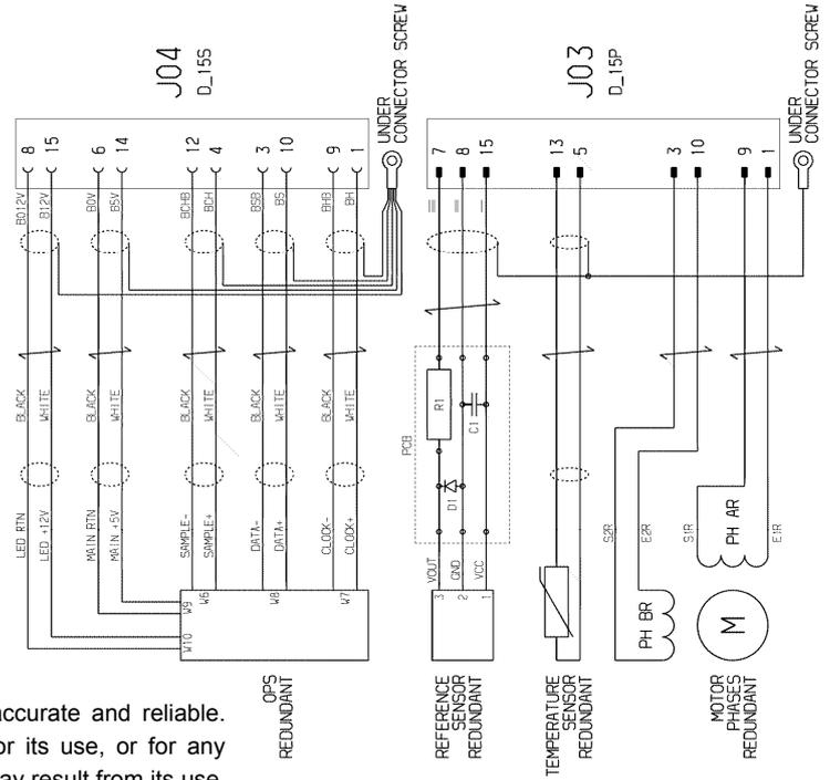
Figure 5: SEPTA 33CS Housekeeping interfaces
