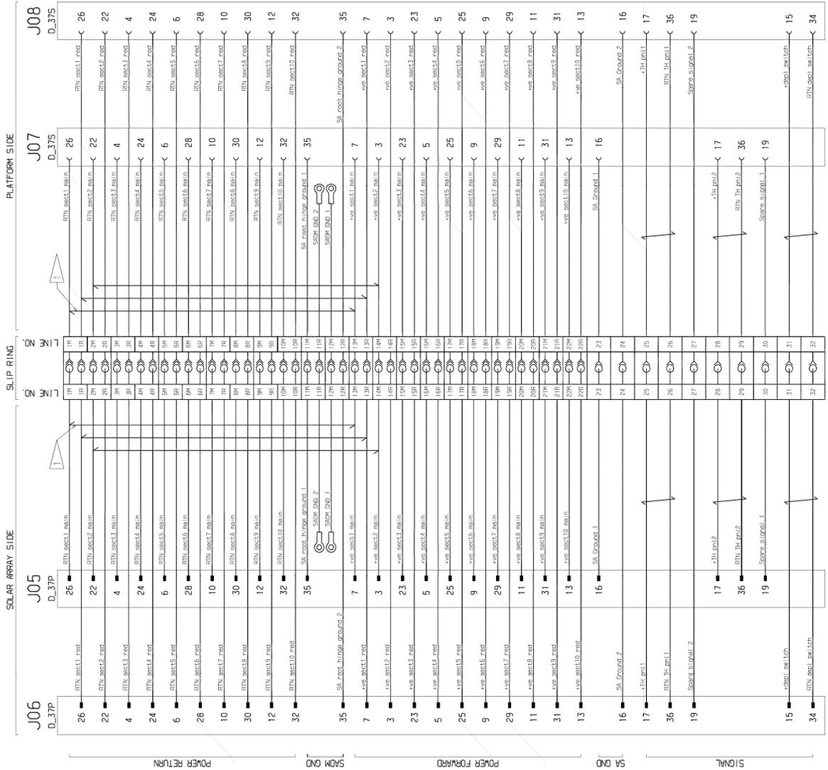
Figure 5: SEPTA 33 electrical transfer scheme
