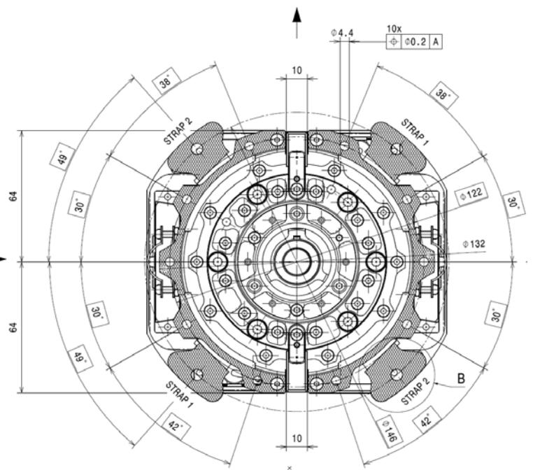
Figure 3: SEPTA<sup>®</sup>33 Spacecraft Interface view
