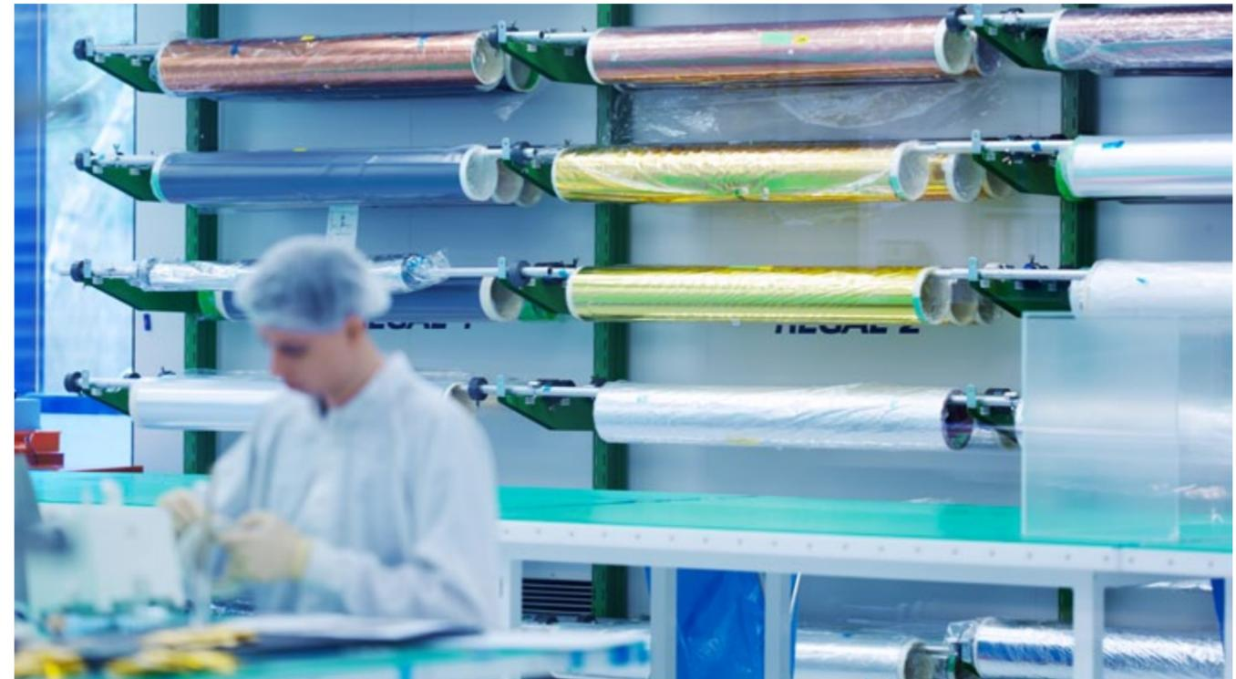
Our production processes for the cutting of blankets, electrical grounding and assembly of multi-layer insulation, velcros/stand-offs, attachments and advanced cleanliness are proven by many tests and several flight heritages. Advanced solutions have been worked out e.g. for high temperature multi-layer insulation around thrusters with Titanium foils, mechanism multi-layer insulation.
