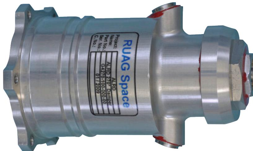
The Viscous Deployment Damper essentially consists of housing and rotor. When turned, the rotor forces highly viscous working fluid through narrow gaps. The resistive torque thus generated is proportional to shaft angular rotation rate and fluid viscosity. The damper thus eliminates the need for high ratio gears and their corresponding mass and friction.
