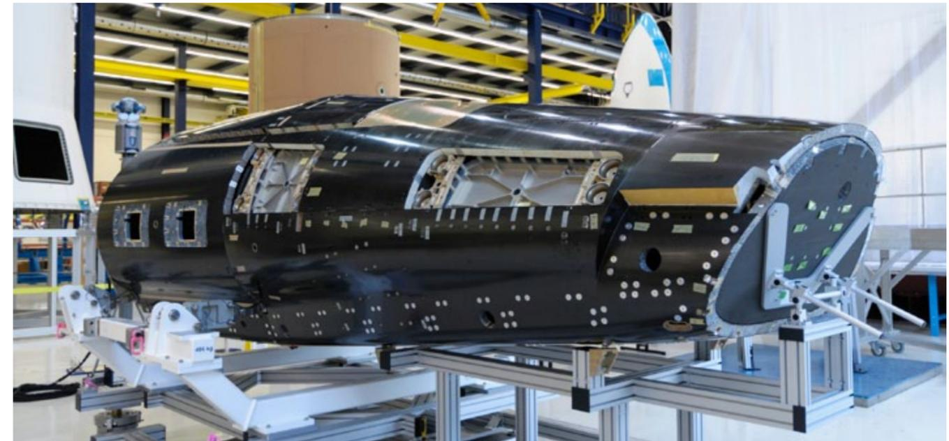
The backbone of every spacecraft is a lightweight structure that holds different types of equipment including the mission's payload, avionics, propulsion and power subsystems in place. Aluminum panels with integrated heat pipes as well as CFRP panels in free form shapes are fully designed manufactured and tested at RUAG Space.
