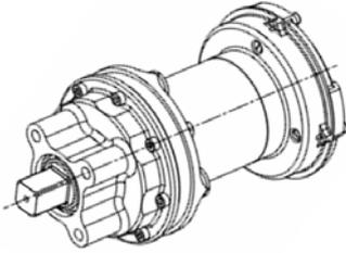
Figure 1: 3-D view of the Eddy Current Damper
