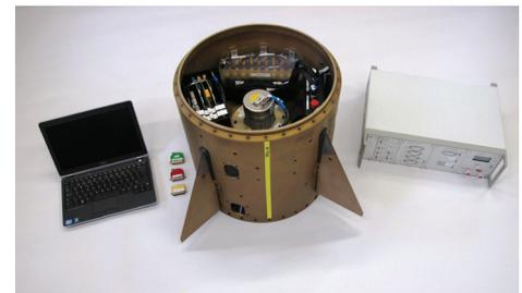
An S19 family system with its electrical ground support equipment
